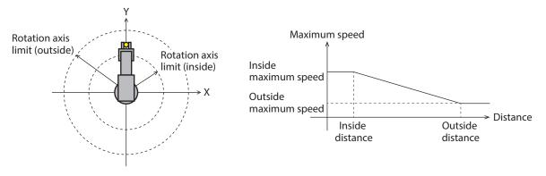
• Set a value greater than the "Rotation axis limit inside distance" parameter to the "Rotation axis limit outside distance" parameter. If the value set in the "Rotation axis limit inside distance" parameter is greater, the limit function is disabled.
