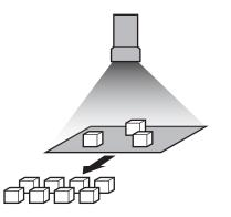
Pickup of loads that have been placed in a random position on the pallet
