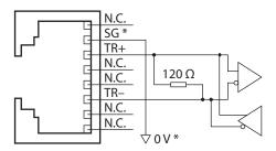
\* SG is electrically isolated from the power ground of the CN1 connector.
