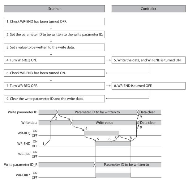
\* If an error occurs while data is being written, the WR-END and WR-ERR are simultaneously turned ON.
