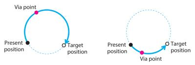
When the radius of the circular arc connecting the present position, via point, and target position is larger than the upper limit value (2,000 mm), or when the present position, via point, and target position are on the same straight line, operation is not started and information of Operation start error is generated.
