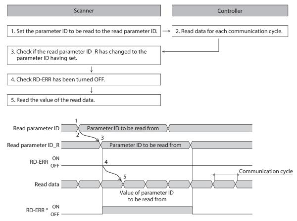
\* If the parameter ID out of the setting range is set to the read parameter ID, the RD-ERR is turned ON at the same time when the read parameter ID\_R is updated.
