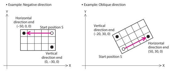
If the Z coordinate for the horizontal direction end and/or the vertical direction end, the path inclined in the Z direction can also be specified. It is the coordinates on a plane that includes the horizontal direction end and the vertical direction end having set.
