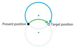
Set a value to "Radius" so that a value of twice the radius is equal to or greater than the linear distance between the present position and the target position. If this condition is not satisfied, or if the present position is equal to the target position, operation will not start and information of Operation start error will be generated.
